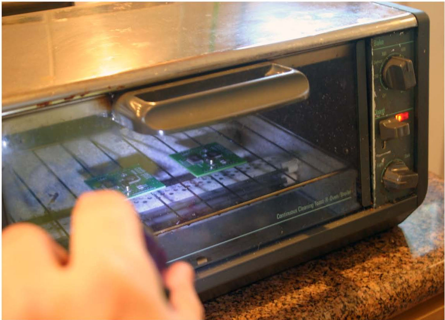
Using an old toaster oven to reflow the solder
