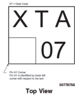
LM358TP micro SMD Marking Orientation
